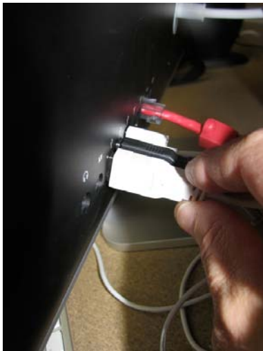
Connecting the cable to a USB port on the back of the computer.
