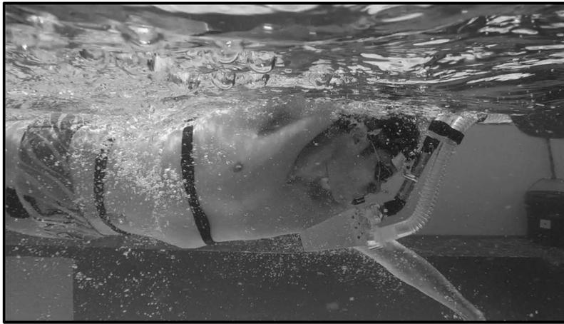
**Figure 2.** The custom built snorkel used for this study. Subjects wore a nose clip and breathed through a mouthpiece connected to a 2-way nonbreathing valve that was affixed to the subject's forehead using an aluminum bracket. A fin was mounted to the base of the snorkel to stabilize the snorkel in the water.
