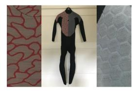
Figure 1. Left: graphene synthetic fleece material (red). Center: Hurley 2-mm full-suit back zip wetsuit turned inside out showcasing graphene-infused nylon fleece on the left aspect of the torso (red/gray) and traditional polyester fleece on the right aspect of the torso (grav)
