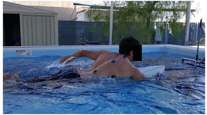
**Figure 2** — Instrumented subject paddling a shortboard in the swim flume without a vest.
