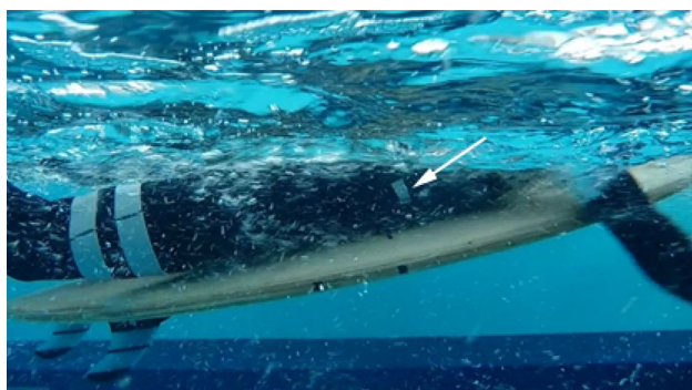
Fig. 2 Under water view of the surfer's position while paddling a surfboard in the swim flume. Two markers on the side of the board were used as a linear scale. The marker on the subject's torso (denoted with arrow) was used to determine position on the board
