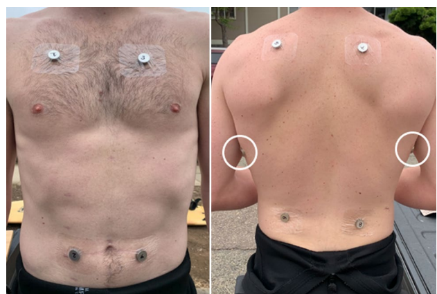
Fig. 1 Thermistor placement for field and laboratory studies. Note sensor placement over the lateral aspect of the scapula in the right pane
