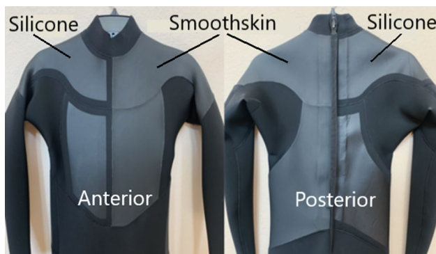
Fig. 2 Anterior and posterior view of custom designed 2 mm experimental wetsuit
