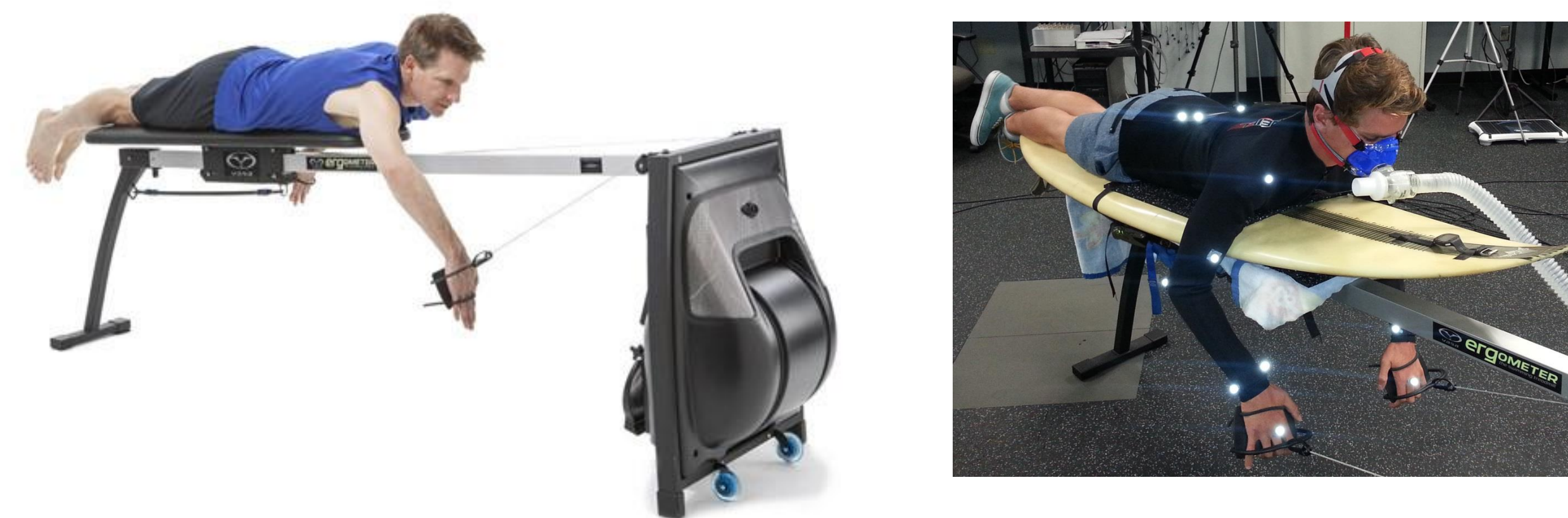
Figure 1 Vasa Inc. swim bench ergometer (left), experimental setup (right). Subjects did not wear a wetsuit in either paddling condition.
